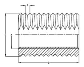
Female thread A = M3 Length B = 6 Male thread E = 5.0Min hole depth blind hole = 7
